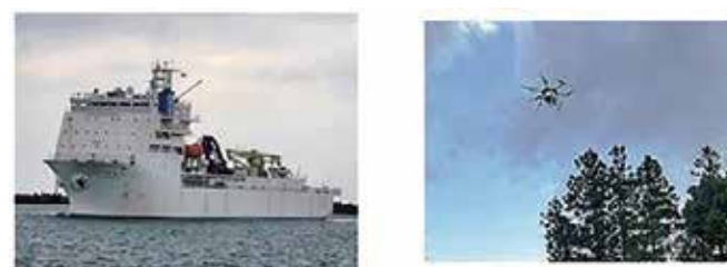
Figure 4: Shipboard base station and wire-powered drone base station
