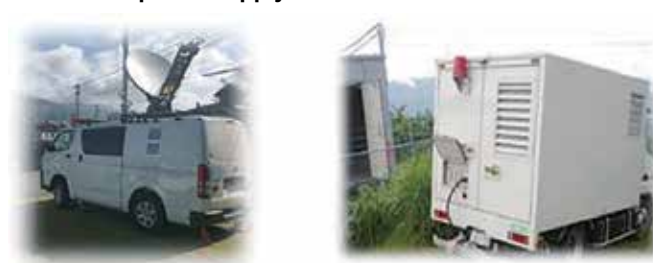
■ Figure 3: Vehicle-mounted base station and mobile power supply vehicle
