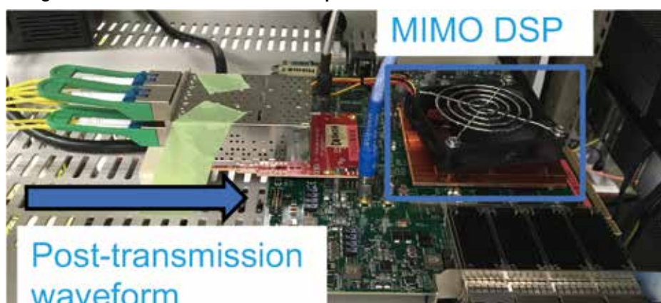
■ Figure 3: Real-time MIMO DSP for coupled 4-core fiber
