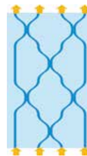
■ Figure 8: Example configuration of an arbitrary mode-control device in a repeater
