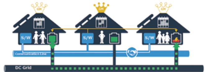
■ Figure 2: Autonomous distributed control of household power supply by APIS
