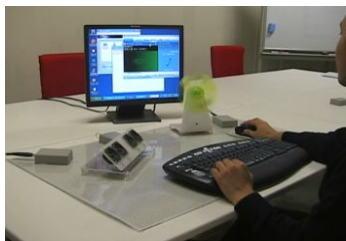
PC peripheral equipment on signal and power by wireless
