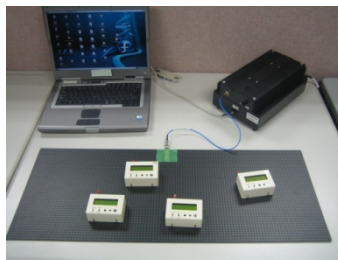
Sensor network with Wireless Power and Data Transmission
