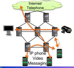
Dependable mesh system usable in both normal and emergency situations
